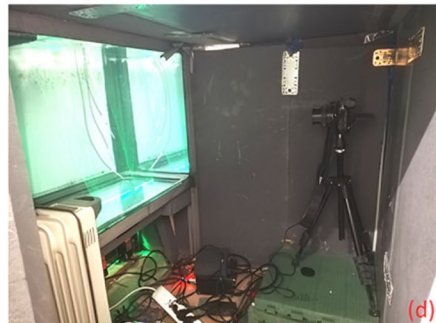
Fig. 1 Schematics a, b and pictures c, d of the experimental setup: a side view, b top view, c experimental setup in the cold room, d inside of the insulated box with the PIV system
