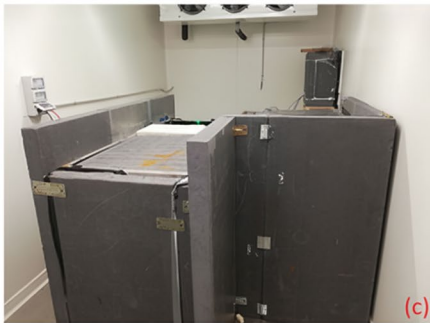
Fig. 1 Schematics a, b and pictures c, d of the experimental setup: a side view, b top view, c experimental setup in the cold room, d inside of the insulated box with the PIV system
