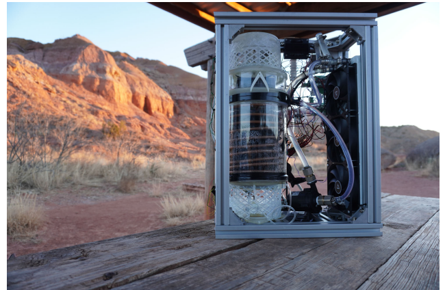
FIGURE 6. Prototype of atmospheric water generator during testing in texas, palo duro state park [4].
