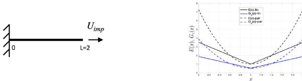
Fig. 1 – 1D benchmark problem (left) and heterogeneous Young modulus and critical energy release rate (right)
