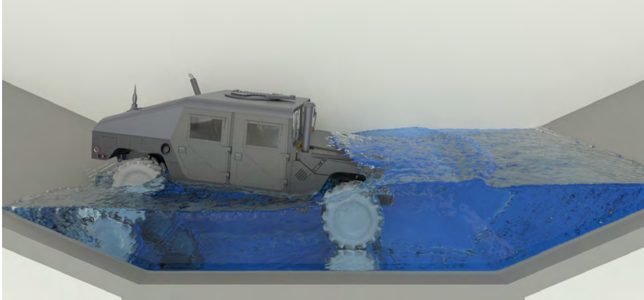
Fig. 7 Vehicle fording simulated using Chrono [34]. In this example, many features of Chrono are displayed, such as rigid body dynamics to simulate the interaction between the various components of the vehicle, flexible body dynamics to simulate the deformation of the tires, and SPH (smoothed-particle hydrodynamics) to simulate the interaction between the fluid and the vehicle body
