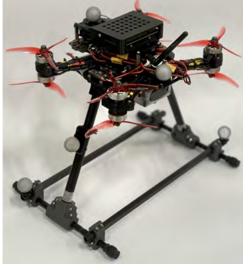
Fig. 3 X8-copter UAV employed to test the flight stack [1] and the accessory files [4]
