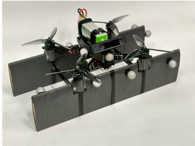
Fig. 4 Quad-biplane UAV employed to test the flight stack [2] and the accessory files [5]
