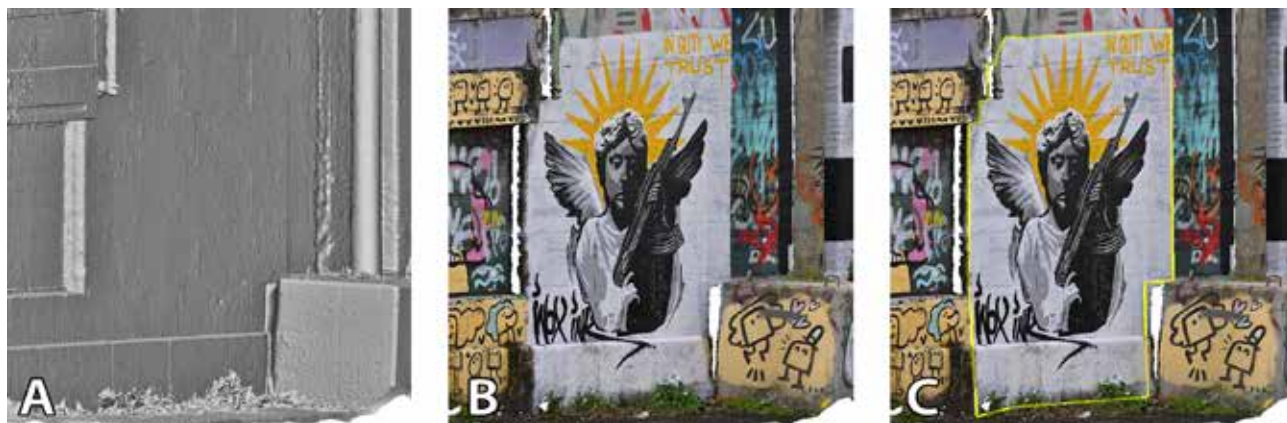
Figure 22. AUTOGRAF can compute a 3D surface mesh (A) with texture (B) from the series of overlapping photos acquired per graffiti. On this textured mesh, the GRAPHIS image polygon can be projected (C) to yield a 3D closed polyline whose vertices have real-world 3D coordinates.
