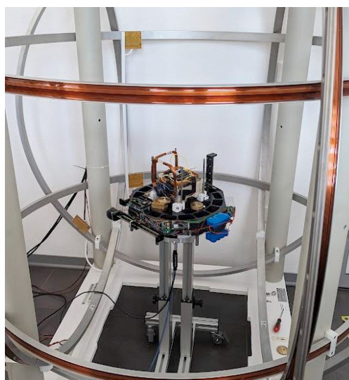
Figure 3: the Cubesat Test Platform on the CubeDyna ABT inside the Helmholtz cage.
