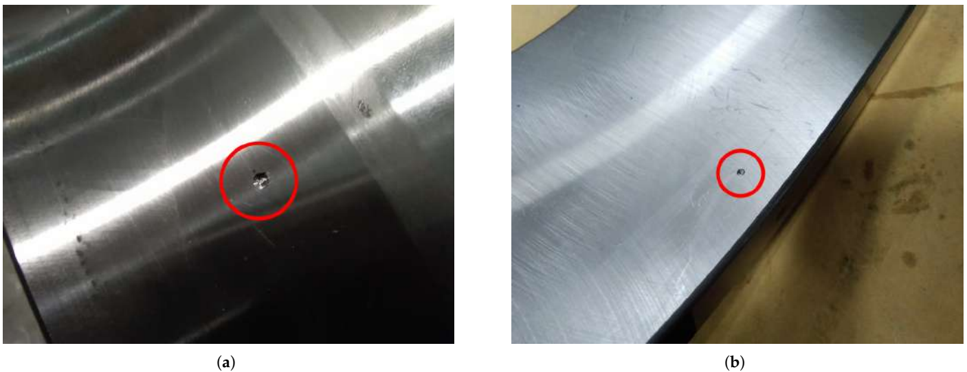
Figure 10. Localized damage: (a) IR damage and (b) OR damage [14].
