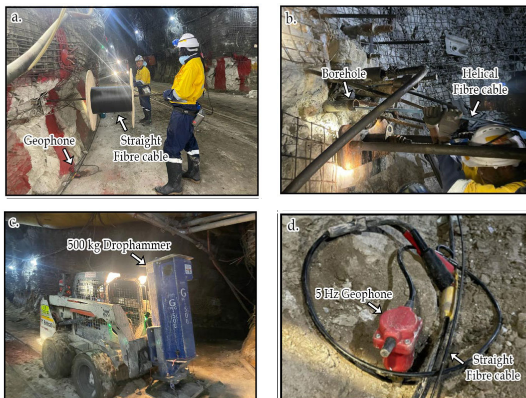
Figure 5—(a) Deployment of straight fibre along the tunnel floor at South Deep mine level 100, (b) Helical fibre cable inserted into the borehole for a length of 67 m. (c) A 500 kg drophammer used as a seismic source in underground tunnels mounted on a skid steer 530 bobcat and (d) Drilled 5 Hz one component geophones placed along the straight single mode fibre optic cable
