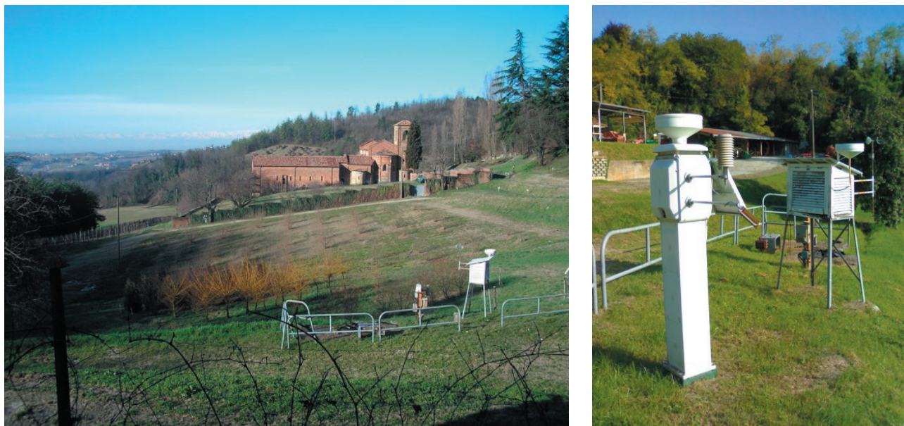
Figure 2. Weather stations at the Vezzolano Experimental Farm: (a) the mechanical station that operated in the period 1961-2005 and, on the background, the Vezzolano Abbey (photo IMAMOTER, 11.03.2009) and (b) the automatic station placed near the older one in 2002 by the Regional Agrometeorological Network (RAM). Stations are placed in the in front of the farmhouse (photo IMAMOTER, 10.05.2008).
