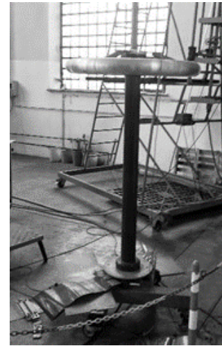
Fig. 2. HAEFELY R600 damped capacitive divider
