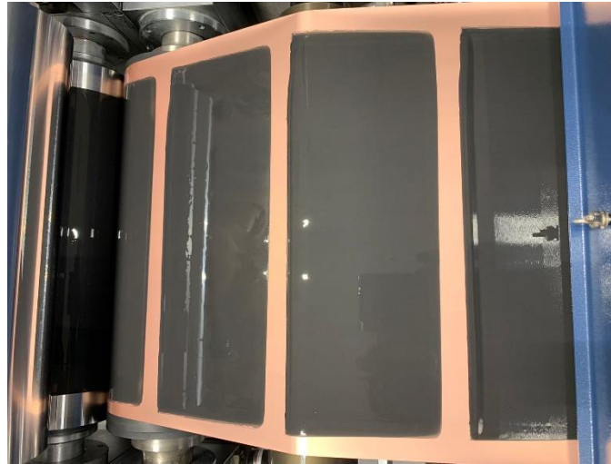
Figure 1. Anode coating on roll-to-roll machine
