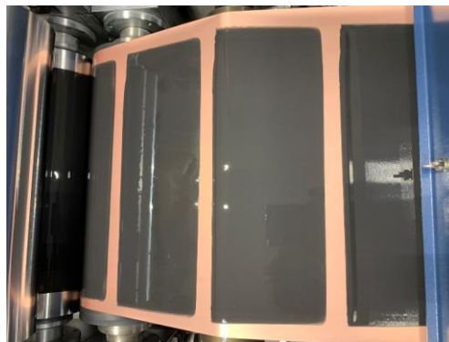
Figure 1 – Anode coating on roll-to-roll machine
