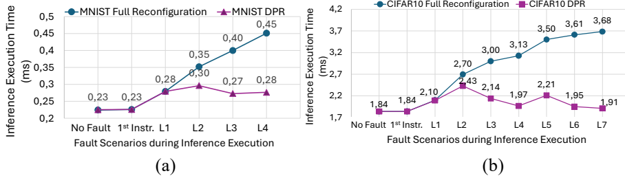
Fig. 7. Total inference execution time considering fault occurrences at different stages of the inference process with and without DPR for MNIST (a) and CIFAR10(b).
