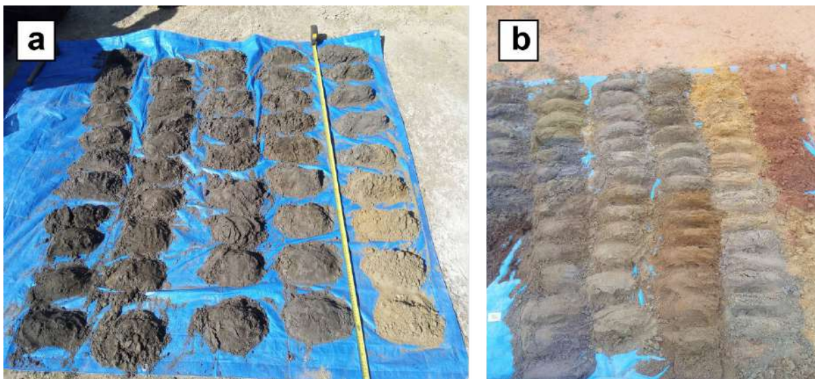
Figure 10. Tailings samples from the a) new tailings storage facility and (b) the old tailings storage facility.
