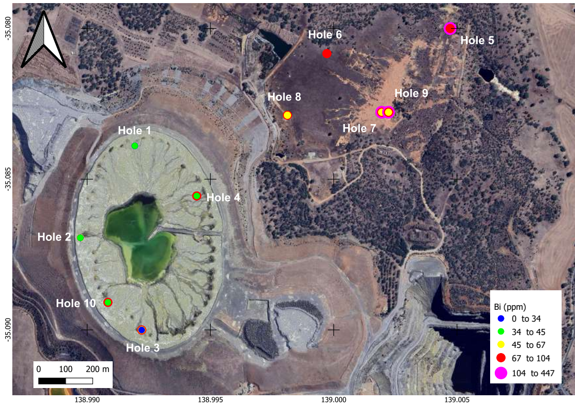
Figure 26. Spatial distribution of highest Bi values (ppm) across the Kanmantoo mine site.
