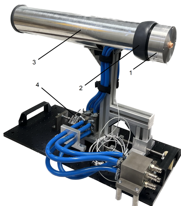
Figure 13. Picture of the final setup: (1) pressure chamber and nozzle model, (2) chamber/body interface or support ring, (3) external body-extension, (4) S-shaped load cell.
