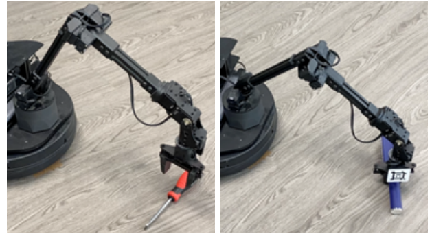
Fig. 8: Two examples of grasp poses for a screwdriver (left) and a hairbrush (right).
