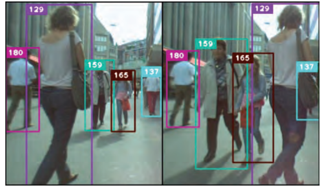
FIGURE 8. Visual demonstration of DeepSORT [141] tracking algorithm in a common crowded situation with frequent occlusion. The algorithm assigns a unique ID to each detected person and consistently maintains this ID throughout the entire tracking process.
