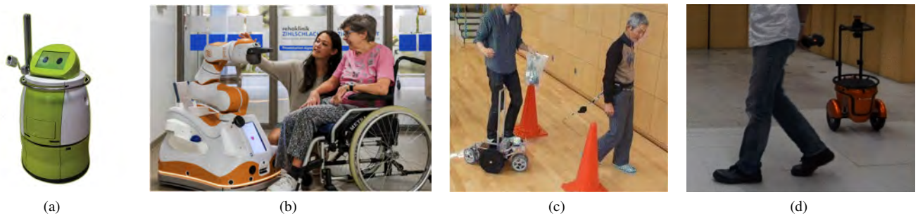
FIGURE 18. Medical assistance robots take on various forms and designs tailored to their specific tasks. For example, Terapio [3], shown in (a), is designed as a medical rounds assistant, while Lio [194] in (b) serves as a caregiver in assisted living facilities. The robots in (c) and (d) are examples of porter robots: the first [161] supports Home Oxygen Therapy, with the tether following system, and the second [123] functions as a home assistant capable of carrying baggage and luggage.
