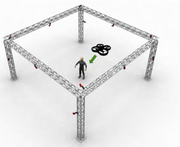
FIGURE 10. An illustration of an indoor multi-camera system, as described in [40]. Within the confines of the setup, both robots and humans equipped with specific markers can be tracked with exceptional precision.
