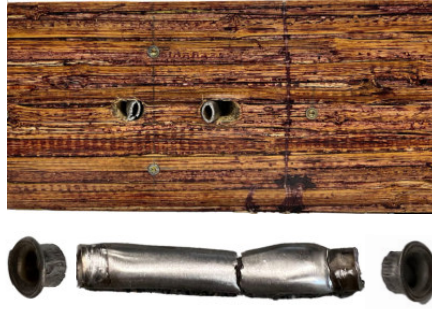
Figure 7: Failure patterns of riveted connections.
