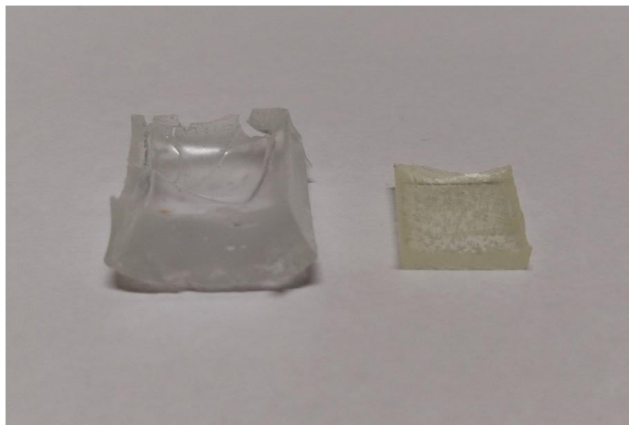
Figure 6. Specimens freshly extracted from toluene ( left ) and dried for three days, completely free of toluene ( right ).
