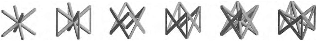
Fig. 1. Lattice cells considered, from left to right: bcc, bccz, fcc, fccz, fbcc, fbccz.
