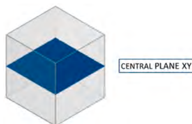
Fig. A1. Representation of the central plane, where stress maps are extracted from
