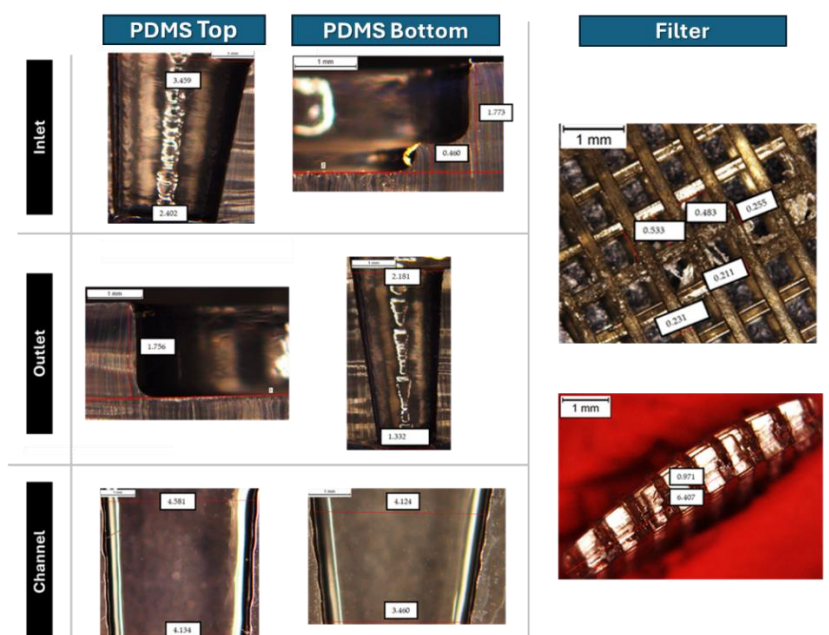
Figure 85: Right: Microscope images of top and bottom layers, with related features measurements. Left: Microscope images of printed filter, with relative features measurements. All measures are in mm. The scale bar is 1mm.
