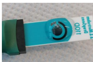
Figure 74: Displacement during the analysis of the analyte and electrolyte solution droplet on the working electrode.
