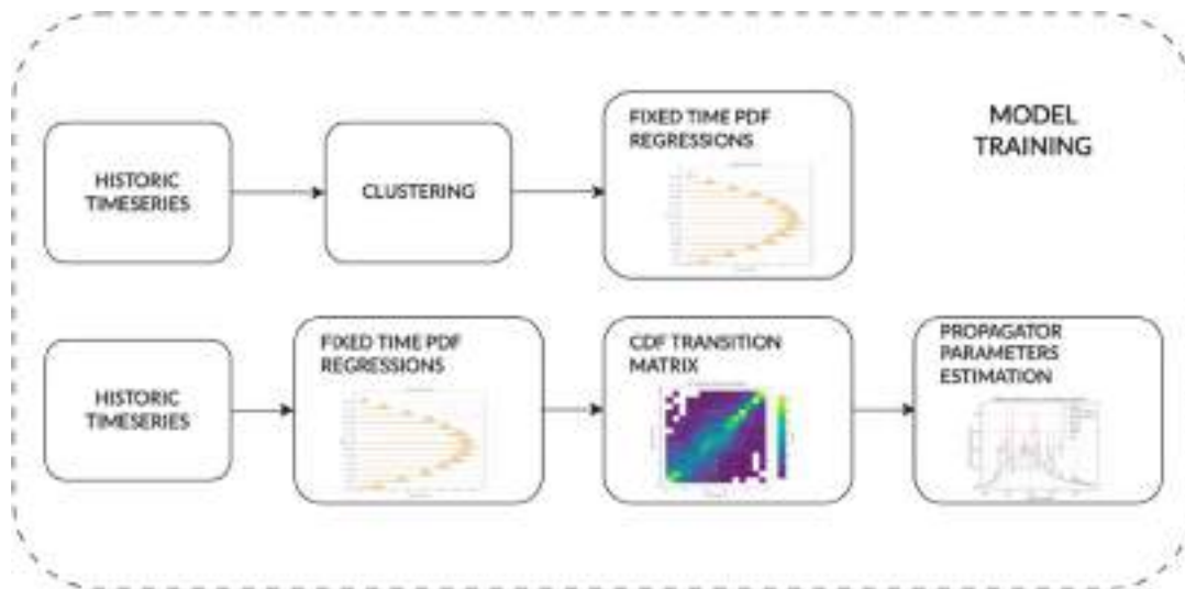
Fig. 2. Training procedure figurative description. Historic data is clustered by month and hour to obtain fixed-time marginal distributions. The same data is then used to calculate its corresponding CDFs with respect to the previously calculated marginal distributions. The CDFs are clustered by month and organized in CDF transition matrices, and fit with a specific solution of the Fokker-Planck equation.
