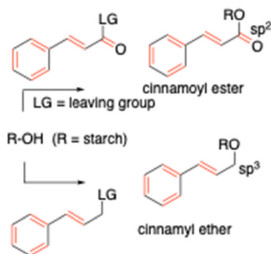
Scheme 1 Acylation and etherification strategies towards cinnamyl starch derivatives (in red the extended conjugated p-system).
