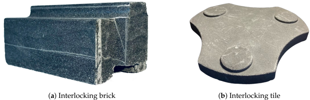
Figure 1. Proof-of-concept designs for interlocking elements made from regolith-rich composite material, demonstrating the feasibility of constructing modular, mortar-free structures using minimal thermoplastic binders.
