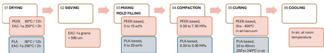
Figure 2. Manufacturing steps for PEEK- and PLA-based samples: The blue boxes indicate the process parameters specific to PLA, highlighting where they differ from those used for PEEK.
