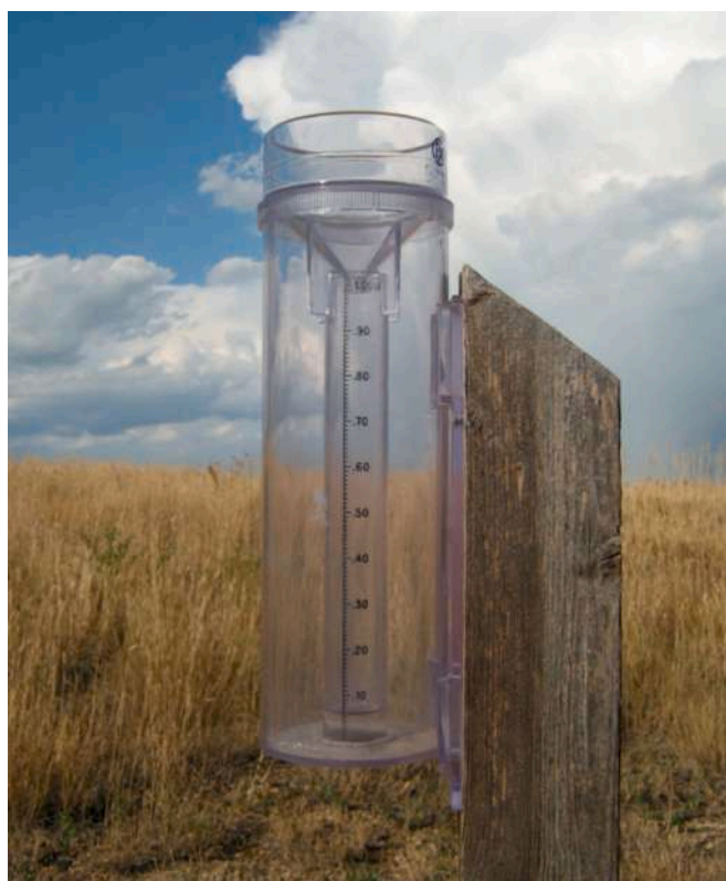
Fig. 22. CoCoRaHS 4-in.-diameter plastic rain gauge-required equipment for each CoCoRaHS observer. The gauge measures to the hundredth of an inch and has an 11.30-in. (287 mm) capacity, with any amount greater than 1 in. flowing into and collecting in the outer cylinder. The funnel and inner cylinder are removed in cold weather for capturing frozen precipitation (Photo by Henry Reges).
