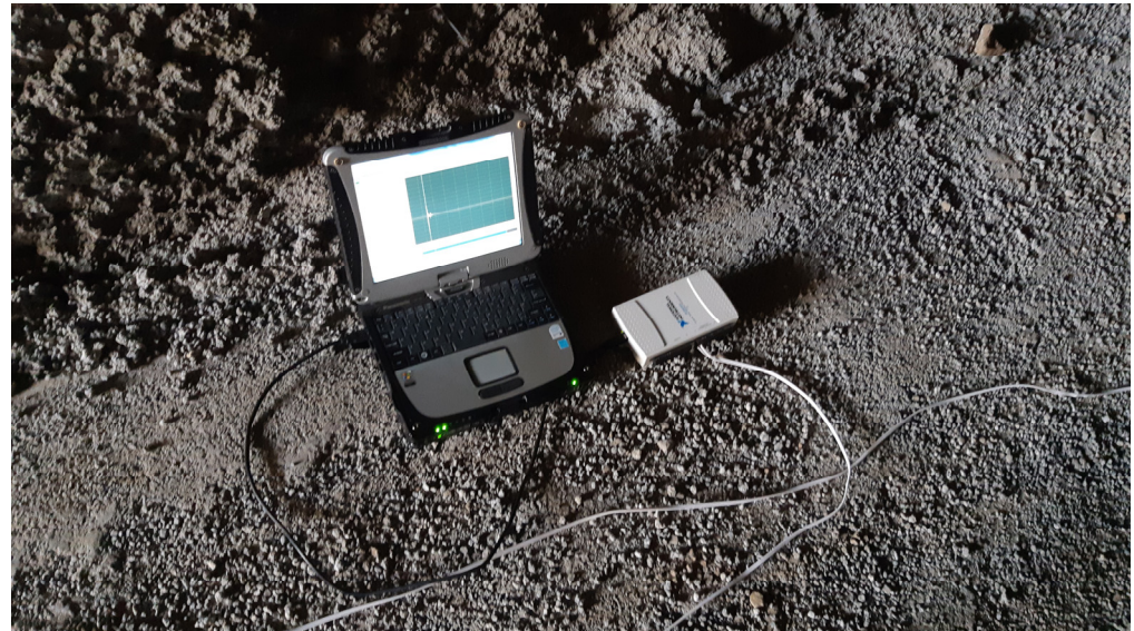
Figure 8. The rugged PC used for the field test and the NI-DAQ card used for the data acquisition. The compactness of the instrumentation is evident for easy handling.
