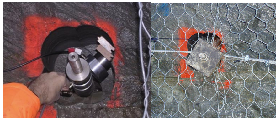
Figure 1. Example of installation with annular cells for tensile loading and a radial cell for transversal loading measurements. (left) during preparation; (right) ready for testing.
