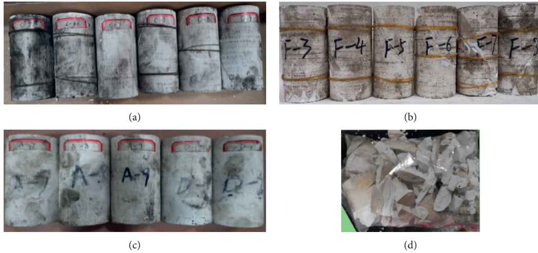
FIGURE 13: Failure modes of triaxial compression of each group of samples. (a) Natural. (b) Dehydration at 45°C. (c) Water saturation. (d) High-temperature dehydration at 220°C.
