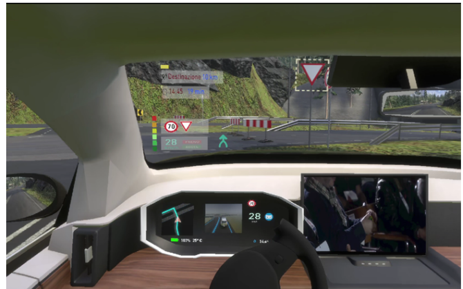
(b) AR-WSD HMI, dashboard and infotainment display devised in this work
