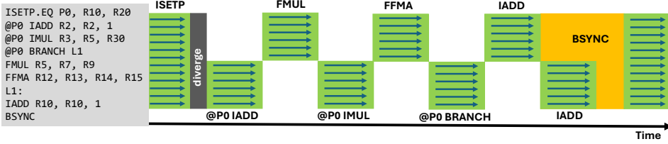
Fig. 5. Illustration of the GPU’s divergence operation using the predicate register P0. In the example, a group of threads with a true value in P0 takes the path of the predicted instructions (i.e., instructions with @P0 modifier), and a second group of threads with a false P0 value executes the non-predicted instructions.
