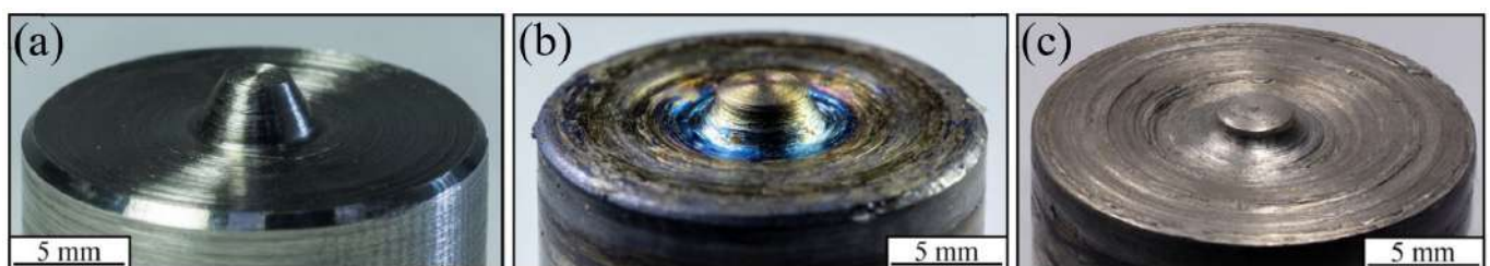
Figure 14. Butt FSW of 2.5 mm thick Ti6Al4V. (a) FSW tool produced from alloy ZhS6U before welding, (b) after ~2 m of welding, and (c) after ~2 m of welding without water cooling ( \omega 340–380 rpm, v 86 mm/min) [162].
