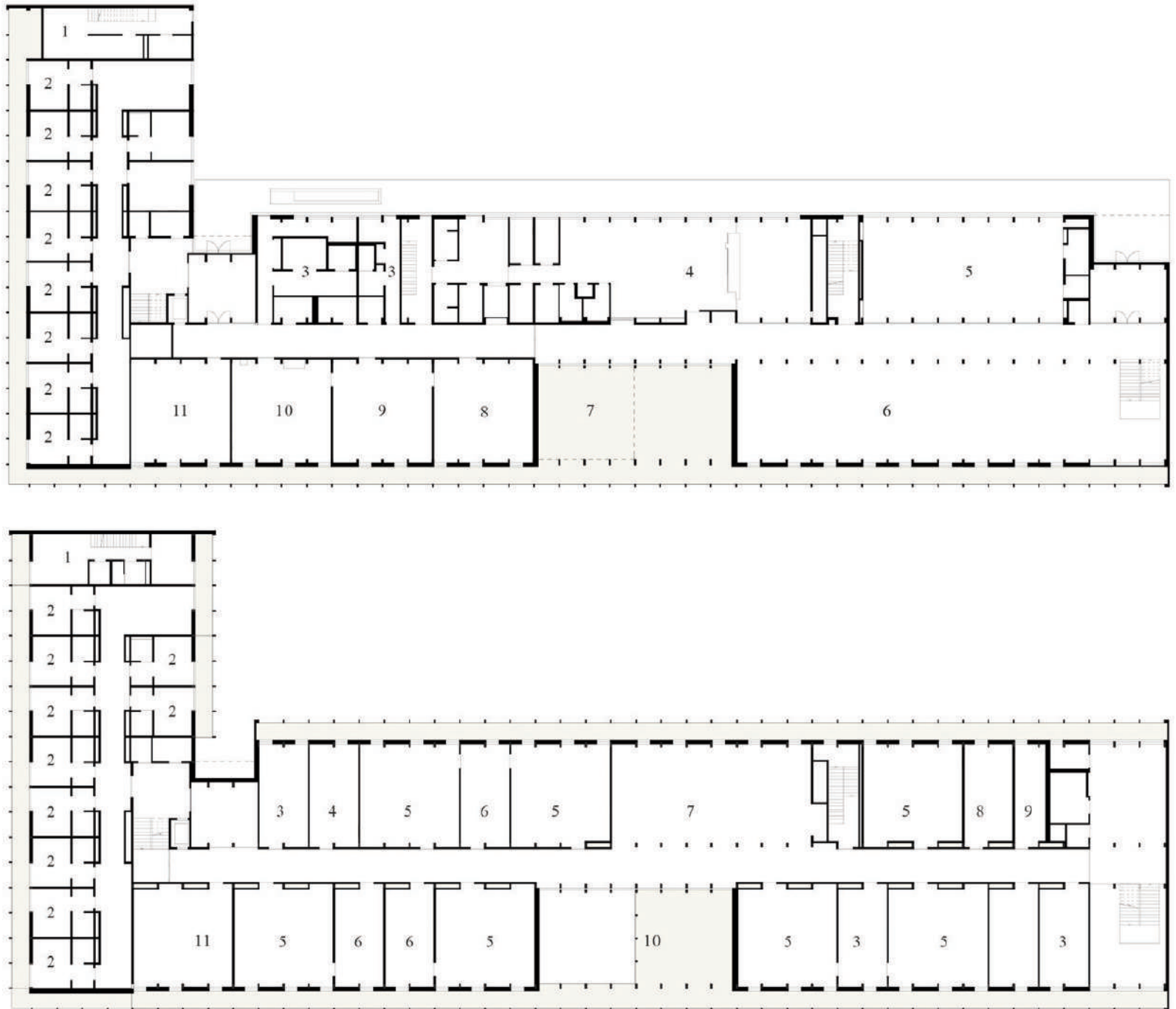
Fig. 4, 5 | Ground floor plan: 1) Hallway; 2) Dormitory room; 3) Dressing room; 4) Kitchen; 5) Auditorium; 6) Canteen; 7) Terrace; 8) Lounge; 9) Didactic kitchen; 10) Classroom; 11) Gym. First-floor plan: 1) Hallway; 2) Dormitory room; 3) Technical room; 4) IT room; 5) Classroom; 6) Group room; 7) Lounge area; 8) Men's toilet; 9) Women's toilet; 10) Terrace; 11) Lounge (credits: A. Senn, 2024; adapted by the Authors).
