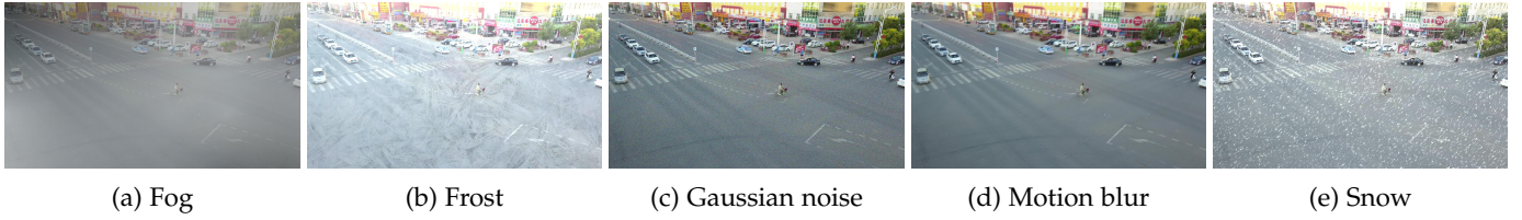
Fig. 7: The selected corruption effects are applied on the same test image using the minimum severity (0).
