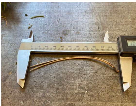
Fig. 1 Pine needle used as fiber-reinforcement for ice
