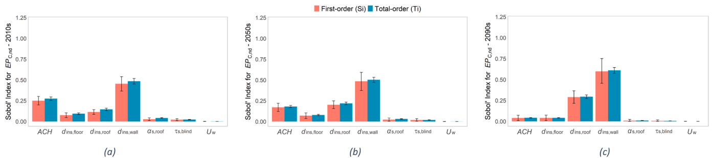
Fig. 6. First and total order of the Sobol indices of the input parameters for thermal energy need for space cooling in the 2010s (a), 2050s (b), and 2090s (c).
