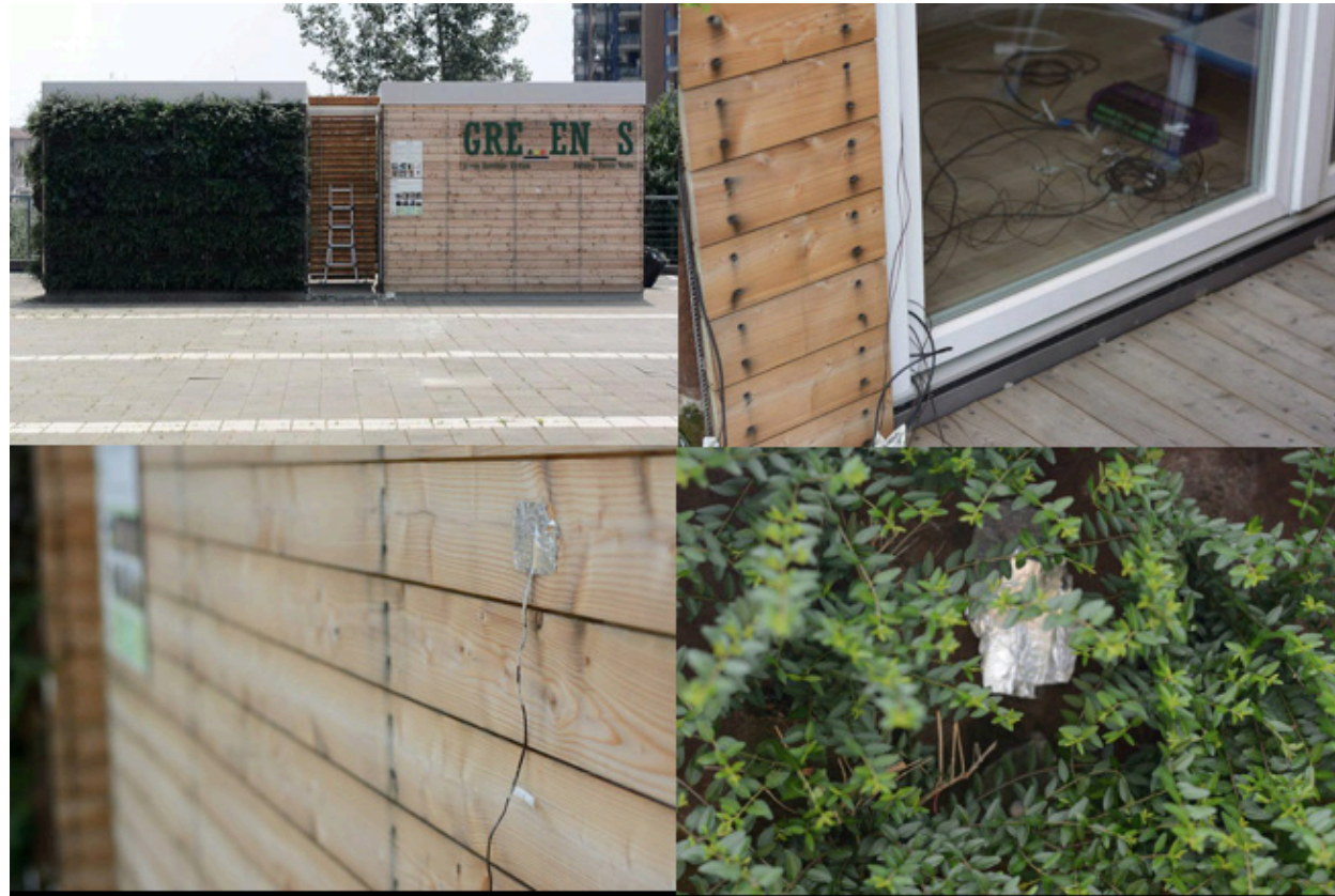
Figure 5. The GRE_EN_S sample building is located in Turin (I). Latitude: 45°04'13". The picture shows the building's surface temperature sensors.
