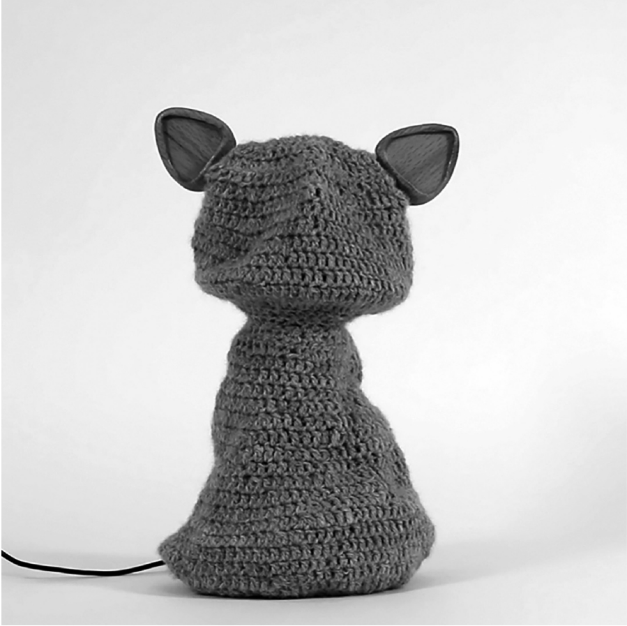
FIGURE 6.1 The Blossom robot displaying a hand-crocheted wool cover and handcrafted wooden ears. These materials were intended to aesthetically fit in domestic environments, be warm to the touch, and evoke a sense of a unique time and place.
