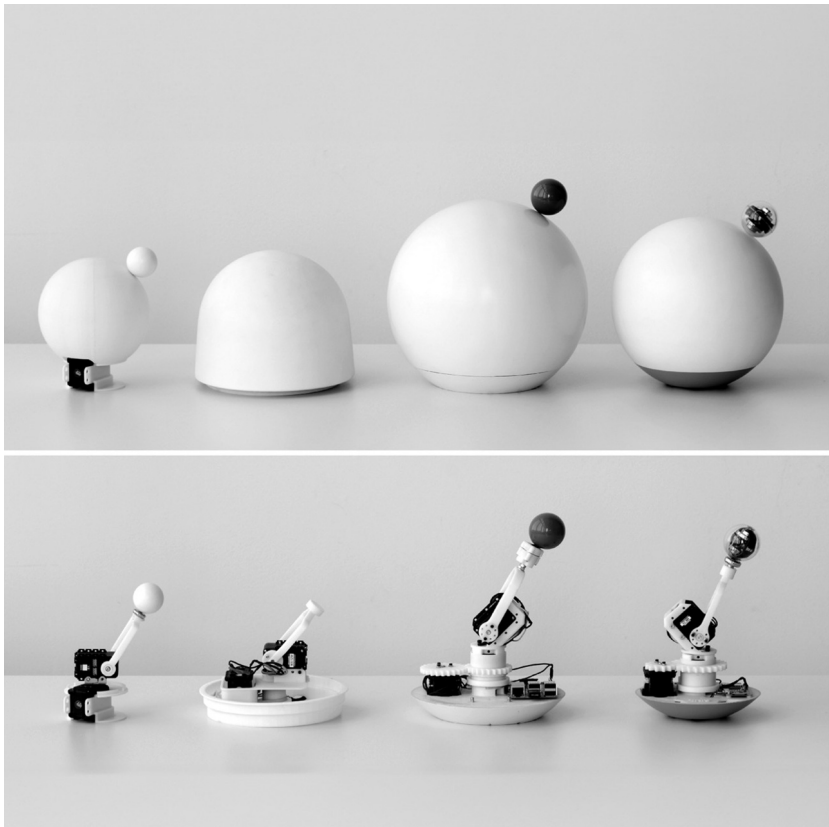
FIGURE 2.4 The greeting machine, prototypes, and mechanisms.
