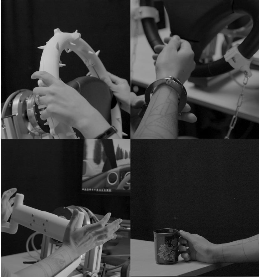
FIGURE 5.6 The four contestational steering wheels developed in the Steering Stories project. Top left: steering wheel with spikes representing full manual driving. Top right: steering wheel with handcuffs representing traded control driving. Bottom left: game-like handles to steer, representing shared control driving. Bottom right: no steering wheel representing full autonomous driving.
