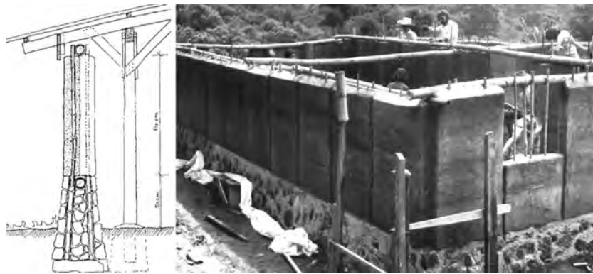
Fig. 1. Bamboo/Earthquake-resistant prototype building, Alhué, Chile, 2001 (5) A reference here (?).
