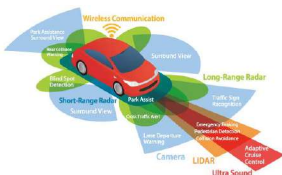
Fig. 7. Smart sensor systems implemented in the autonomous car
