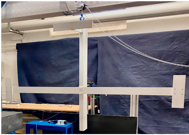
(a) Large steel aircraft with end winglets (#1).
