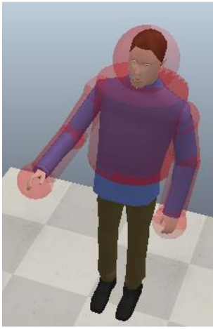
FIGURE 9 OPERATOR SCHEMATISATION USING SIMPLE GEOMETRY VOLUMES
