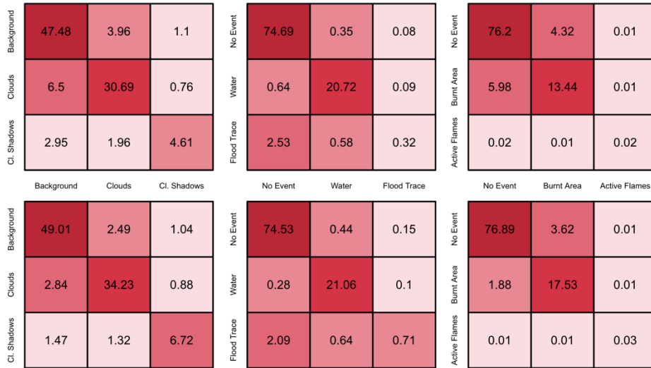
Fig. 4. Confusion matrices of segmentation tasks reporting the absolute percentage value of true and predicted classes. Columns of two matrices from left to right indicates: clouds segmentation, floods segmentation and fires segmentation. Rows of matrices from top to bottom indicates: SSL configuration, SL configuration.
