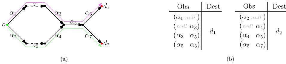
Fig. 2. (a) Graph \mathcal{G} and 2-legible (o, D) -connecting walks \mathcal{P} = \{\gamma_1, \gamma_2\} , with \gamma_1 depicted in violet and \gamma_2 depicted in green. (b) Goal recognition function \Omega^{(2)} that associates each sequence of observations of length 2 with its corresponding destination. The observer, by consulting this mapping, can tell where the actor is going after making two observations. (For interpretation of the colors in the figure(s), the reader is referred to the web version of this article.)
