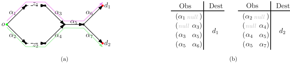
Fig. 2. (a) Graph G and 2-legible (o, D) -connecting walks P = \{\gamma_1, \gamma_2\} , with \gamma_1 depicted in violet and \gamma_2 depicted in green. (b) Goal recognition function \Omega^{(2)} that associates each sequence of observations of length 2 with its corresponding destination. The observer, by consulting this mapping, can tell where the actor is going after making two observations. (For interpretation of the colors in the figure(s), the reader is referred to the web version of this article.)
