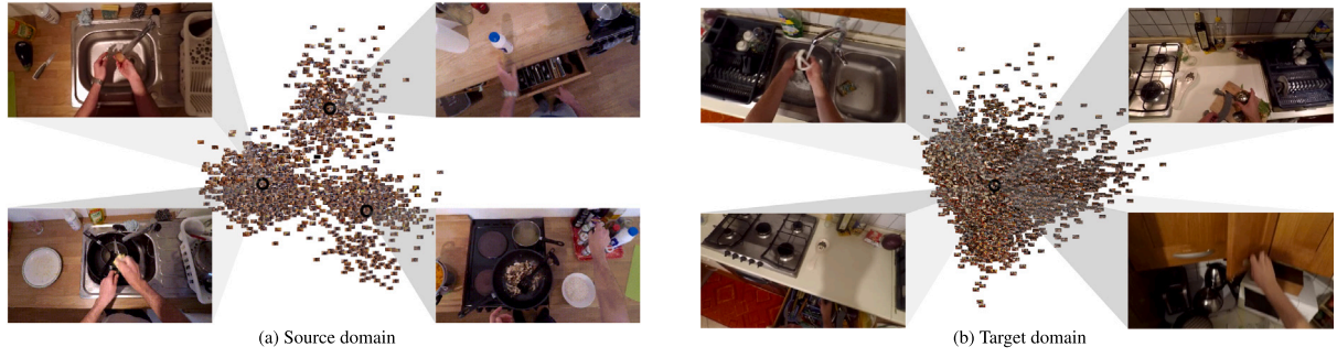
Fig. 2. Feature space of an EAR model. On the left (Fig. 2(a)), the features obtained from a model trained and tested in the same environment are well separated based on the location where the actions are taking place. On the right (Fig. 2(b)), when the same model is used in a different environment, this clustering effect is not present anymore and different locations are mapped to the same region of the feature space.
