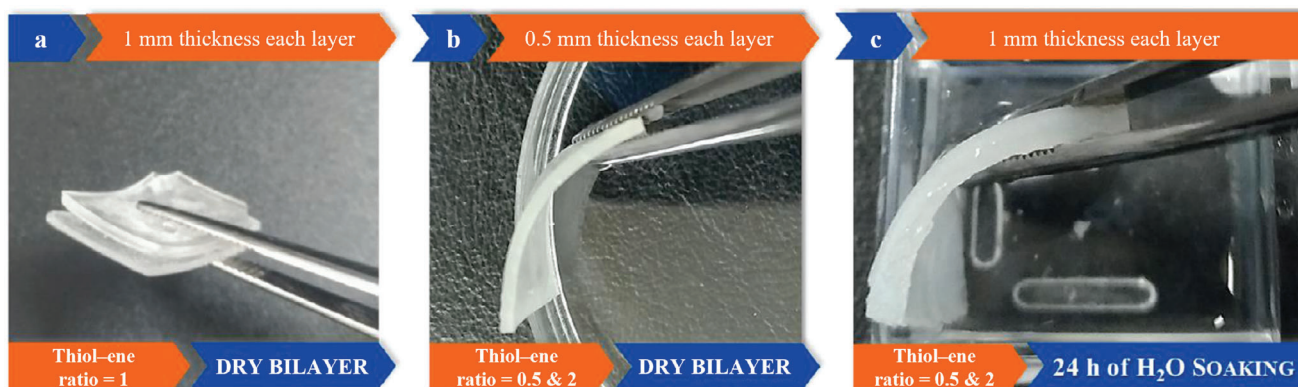
Figure 6. Fluorinated bilayer structures: a) when using stoichiometric polymers no adhesion; b) when combining the off-stoichiometric polymers good adhesion after the photopolymerization reaction c) adhesion is maintained after 24 h of water immersion at RT.
