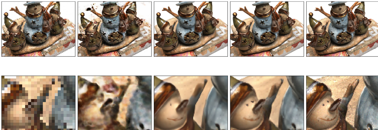
FIGURE 2. DTU scene 3 with 4× scale factor. From left to right: LR nearest neighbours interpolation (19.31 dB), NeRF-SR (19.75 dB), BSRT (23.60 dB), EpiMISR (24.43 dB), HR ground truth.
