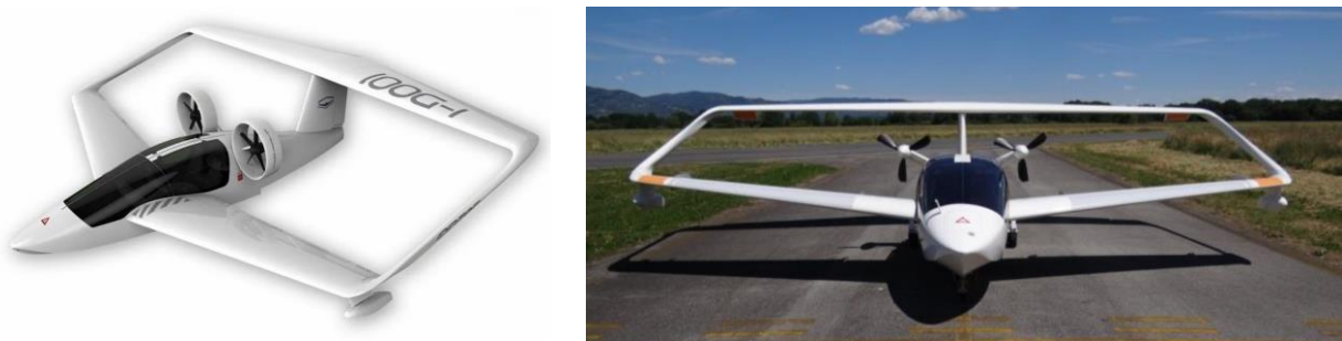
Figure 26. IDINTOS ultralight amphibious aircraft
