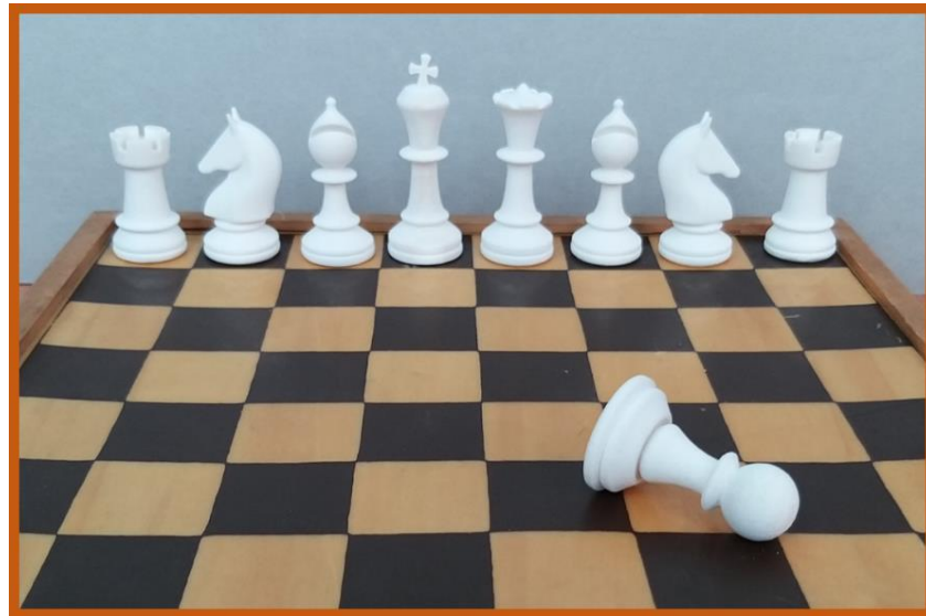
Figure 3. 3D printed chess-like pieces realized via SLS using PA12.
