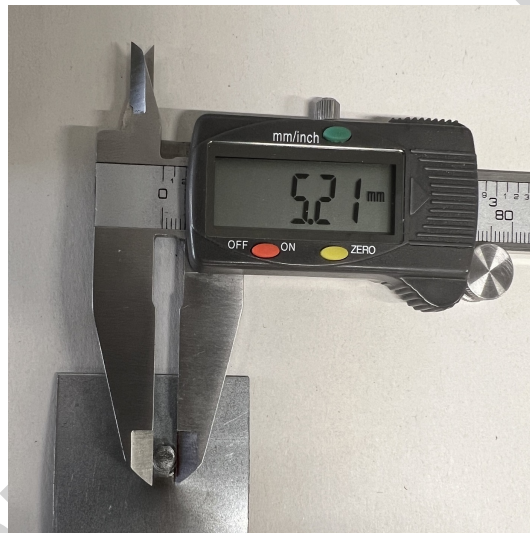
(b) Weld diameter measurement, after shear tension test.
